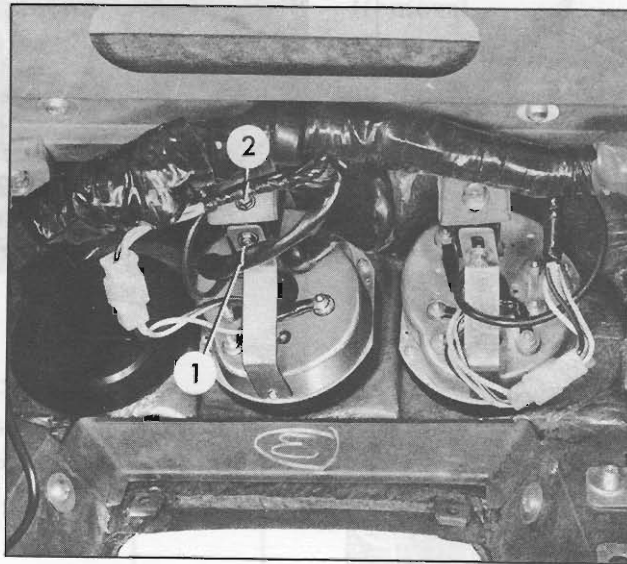
Fig. BE-21 Removing ammeter and fuel gauge
