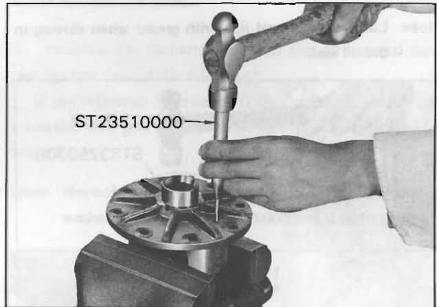
Fig. PD-12 Punching off lock pin
