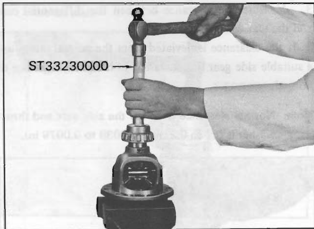
Fig. PD-17 Pressing side bearing cone
