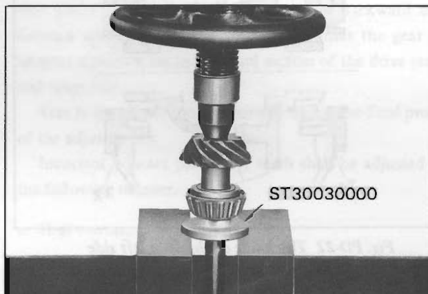
Fig. PD-20 Pressing rear bearing inner race
