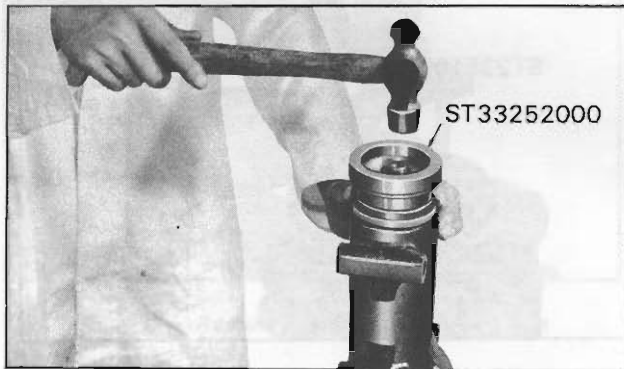
Fig. PD-13 Removing front retainer
