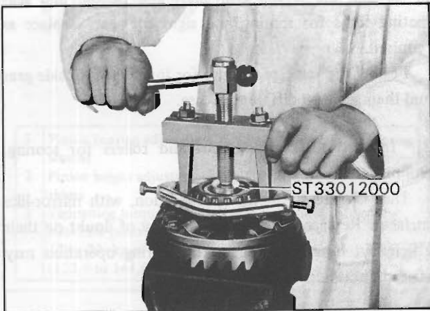
Fig. PD-11 Removing side bearing cone
