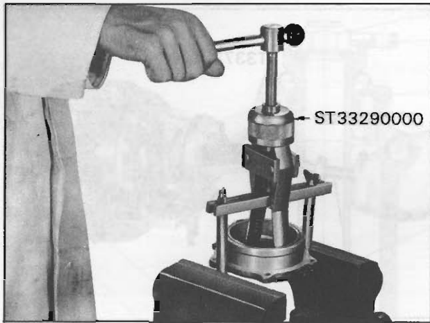
Fig. PD-6 Removing side bearing outer race
