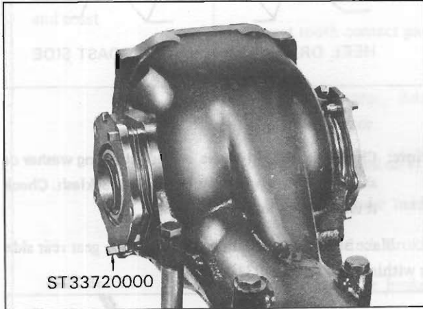
Fig. PD-25 Installation of side retainer
