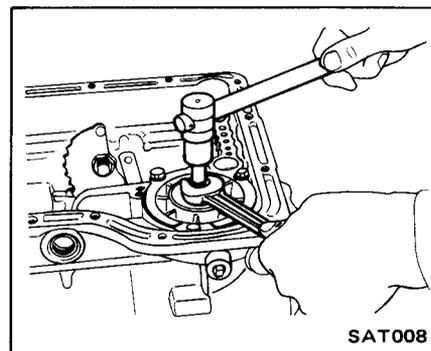
9. Remove input shaft from pump.
