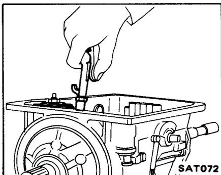
27. Install control valve body. Be sure manual valve is in alignment with selector pin.
