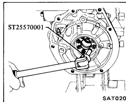
19. Pry off one end of snap ring with a screwdriver. Remove snap ring from low and reverse brake assembly while applying plier force in direction of arrow.
