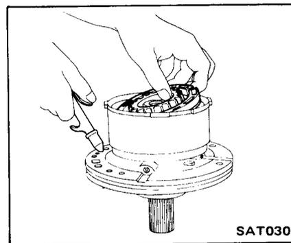
9. Assemble piston, being careful not to allow seal to kink or become damaged during installation. After installing, turn piston by hand to ensure that there is no binding.
