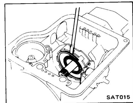
12. Remove brake band strut. Brake band, high-reverse clutch (Front) and forward clutch (Rear) assemblies may be removed together.
