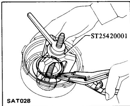
11. Install dish plate with dish facing outward.
