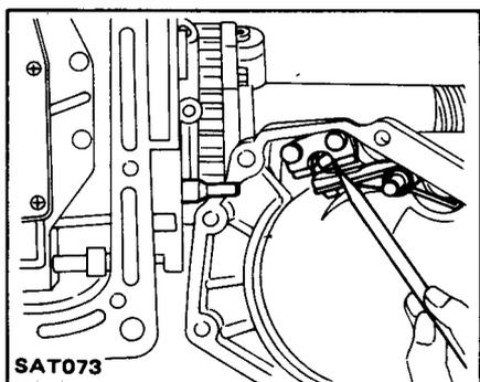
28. Tighten control valve body attaching bolts.
