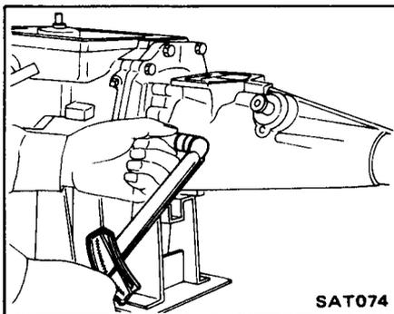
29. Check pump to transmission alignment and install converter housing.
