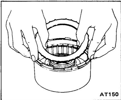
4. Remove spring retainer and springs.
