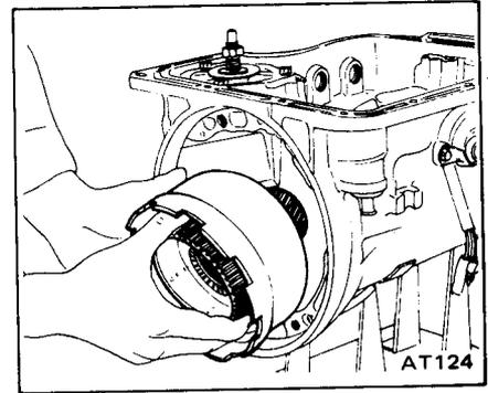
To prevent brake linings from cracking or peeling, do not stretch the flexible band unnecessarily. Before removing the brake band, always secure it with a clip as shown in the figure below.
