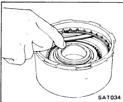
14. Testing high-reverse clutch (Front)
