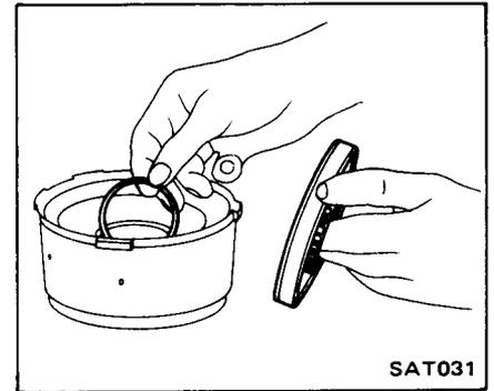
3. Compress clutch springs and remove snap ring from spring retainer.
