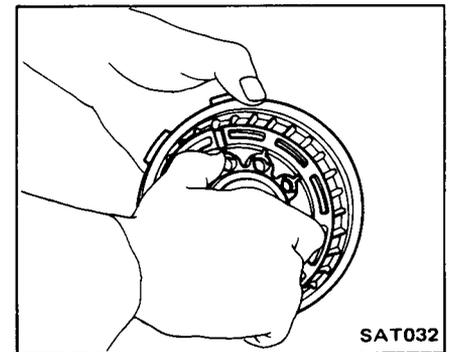
6. Check clutch drive plate facing for wear or damage. Drive plate thickness must not be less than 1.4 mm (0.055 in).
