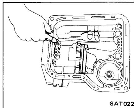
24. Remove governor thrust washer and needle bearing.
