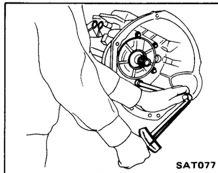
24. Using an air gun with a tapered rubber tip, perform air checks.
