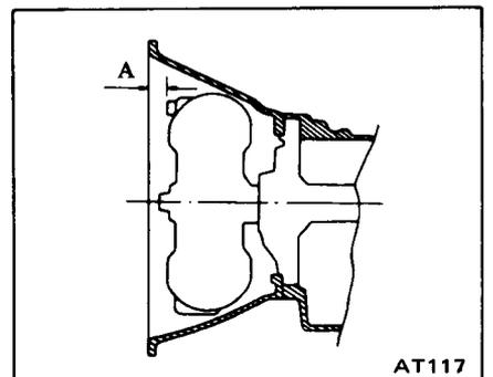
4. Bolt converter to drive plate.
