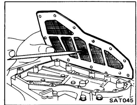
9. Check separator plate for scratches or damage. Replace if necessary. Scratches or score marks can cause oil to bypass correct oil passages and result in system malfunction.
