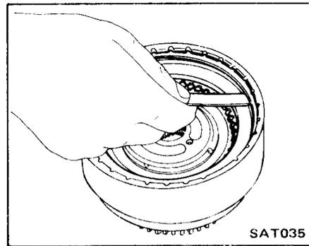
**Test forward clutch (Rear)**
