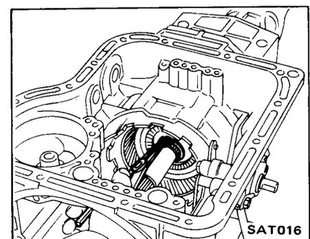
18. Remove rear connecting drum with internal (annulus) gear.
