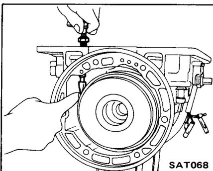
21. Mount oil pump gasket on oil pump with petroleum jelly. Align pump to transmission case and install.
