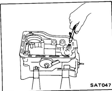
2. Lubricate and install low and reverse piston into the case.
