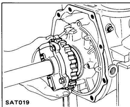
26. Using an air gun with a tapered rubber tip, carefully apply air pressure to remove low and reverse brake piston.
