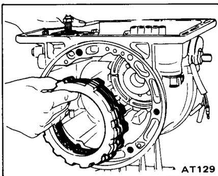
6. After low and reverse brake has been completely assembled, measure clearance between snapping and retainer plate. If measurement exceeds specifications it can be adjusted by replacing retainer plate with one of a different thickness.
