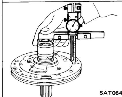
(6) Install thrust washer. Measure from top of oil pump shaft to thrust washer (dimension D).
