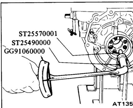
5. Install steel dished plate first, then steel and friction plates, and, finally, retaining plate and snap-ring.
