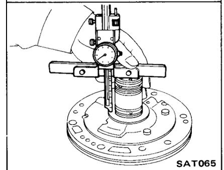
(7) Difference between dimension [A-0.1 mm (0.004 in)-B] and (C-D) is front end play and must be within specified value.
