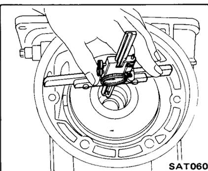
(4) Assemble high-reverse clutch (Front) and forward clutch (Rear) drum assemblies together and lay them flat on bench. Be sure rear hub thrust bearing is properly seated. Measure
