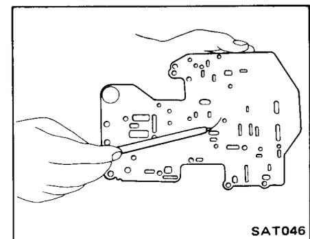
10. Check oil passages in upper and lower valve bodies for varnish deposits, scratches or other damage that would impair valve movement. Check threaded holes and related bolts and screws for stripped threads; replace as needed.
