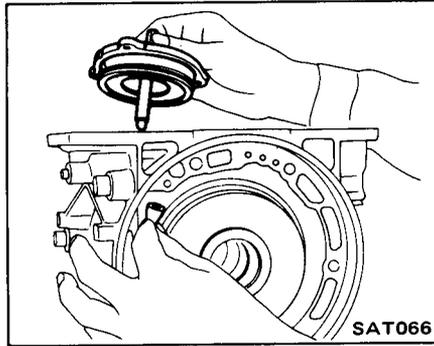
19. Install and torque the retainer bolts. Loosen piston stem.
