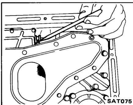
30. Before installing vacuum diaphragm valve, measure depth of hole in which it is inserted. This measurement determines correct rod length to ensure proper performance.
