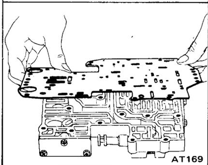
3. During valve body separation, do not scatter or lose orifice check valve, servo orifice check valve, and throttle
