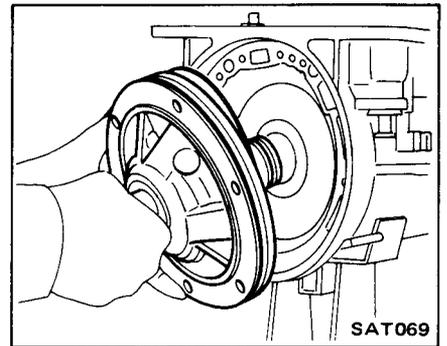
22. Adjust band. Make sure that brake band strut is correctly installed. Torque piston stem to specified value. Back off two full turns and secure with lock nut.
