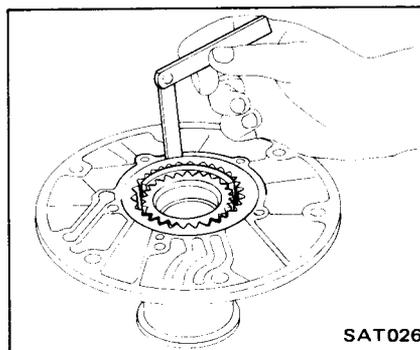
2. Remove pump cover from pump housing.
