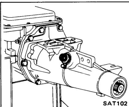
6. Remove oil pan and inspect its contents. An analysis of any foreign matter can indicate the types of problems to look for. If the fluid is very dark, smells burned, or contains foreign particles, the frictional material (clutches, band,) may need replacement. A tacky film that will not wipe clean indicates varnish build up which can cause valves, servo, and clutches to stick and may inhibit pump pressure.
