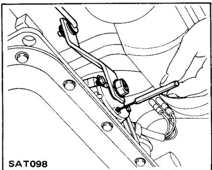
5. Tighten the attaching bolts.
