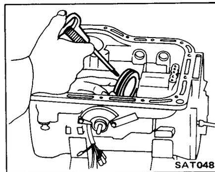
3. Install thrust ring, piston return spring, thrust washer and one-way clutch inner race.
