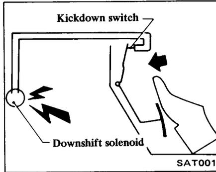
Do not allow the switch to make contact too soon. This would cause
